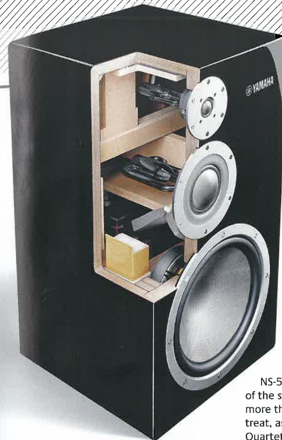
ABOVE: Finished in a luxurious piano black lacquer, the NS-5000's cabinet is fashioned from a laminated white birch plywood. Note 'RS' (Resonance Suppression) chambers behind mid/treble drivers and 'Acoustic Absorber'
